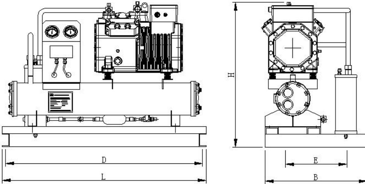
Dimensions of semi-hermetic two-stage piston water-cooled condensing compressor unit:
